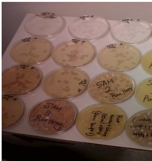
Plate 1. Disc diffusion method used in testing antimicrobial property of honey samples
