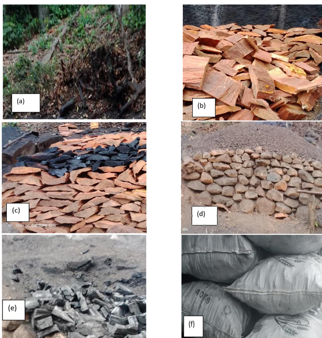
Fig. 2. (a) Forest clearance/logs felled for charcoal production, (b) logs split to desirable sizes (c) splitted logs arranged in the earth pit kiln (d) earth pit kiln are covered by stones at the side and earth on top (e) earth pit kiln opened at the side of stones to exposed ready combusted charcoal (f) bagged charcoal, transported from forest to market
