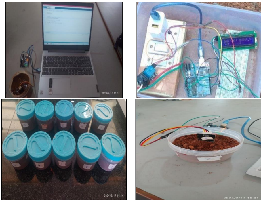
Plate 10. Development of the soil moisture sensor
