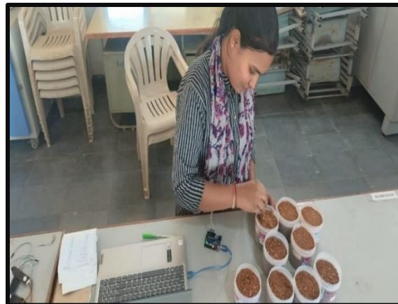
Plate 7. Calibration of sensor in lab
