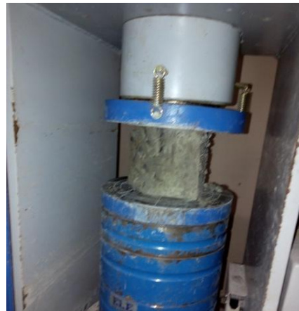
Fig. 1. Compressive strength test of concrete cube
