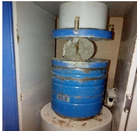
Fig. 3. Split-Tensile testing of concrete cylinder
