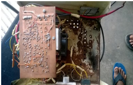
Fig. 17. Packaging of the UPSz into a casing
