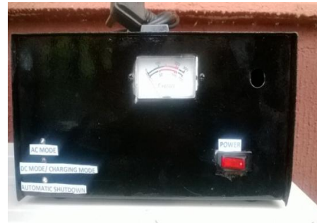
Fig. 19. The Uninterruptible Power Stabilizer
