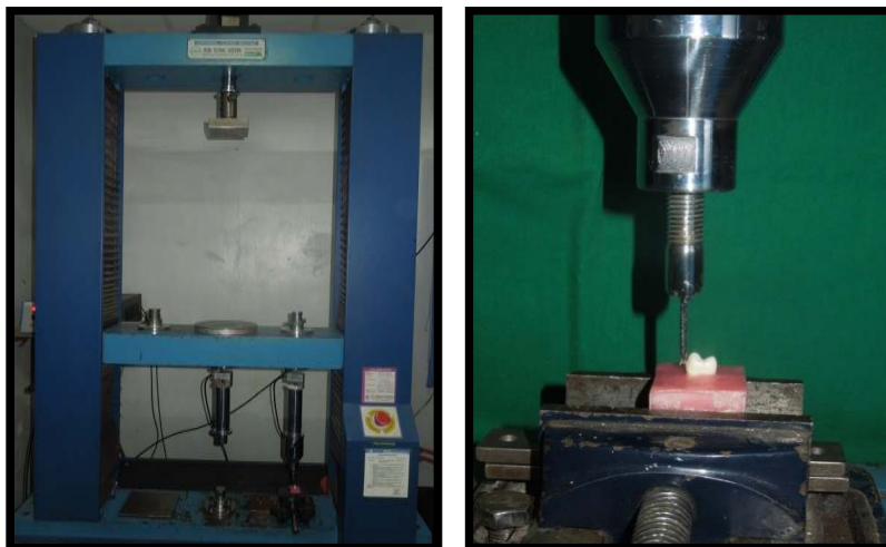
Fig. 6. Instron universal testing machine with a sample
