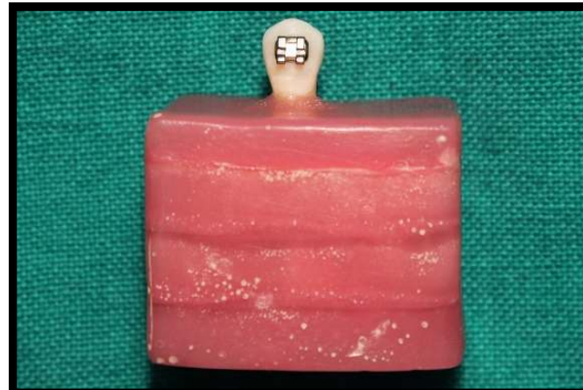
Fig. 5. An extracted premolar with bracket bonded on exposed labial surface
