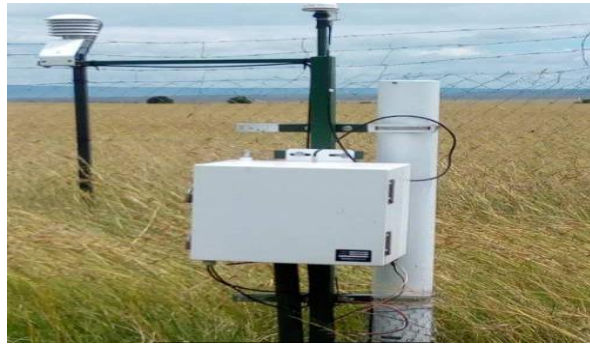
Fig. 2. Installed cosmic-ray soil moisture neutron sensor probe
