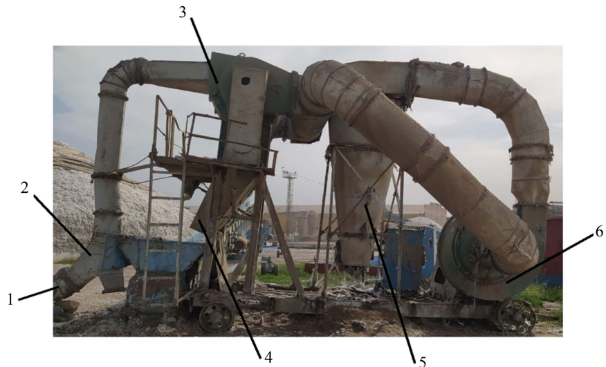
Figure 5. An experimental version of a moving device. 1 inlet pipe, 2 inlets, 3 separators, 4 inclined vibrating mesh surfaces, 5 cyclones, 6 suction blowers.
