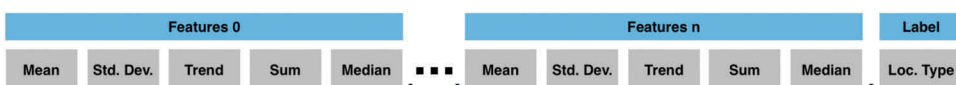
Figure 3. The feature vector is composed by repetitions of mean, standard deviation, trend, sum and median. The last element of the vector is the locomotive type as label.
