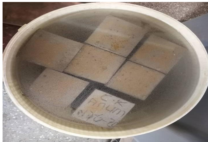
Fig. 3. Cubes in MgSO 4 solution
