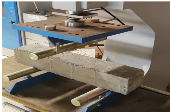
Fig. 2. Concrete beam under flexural strength test
