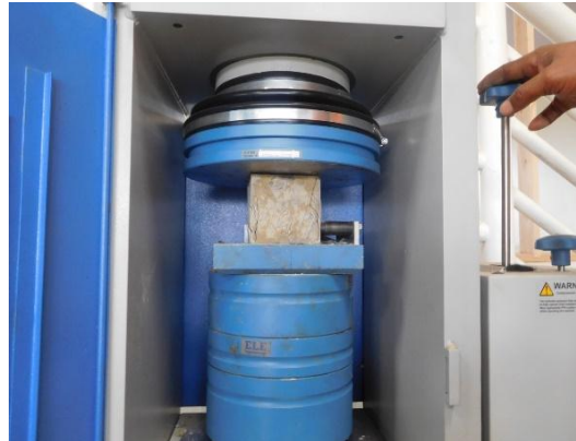
Fig. 1. Compressive strength test setup
