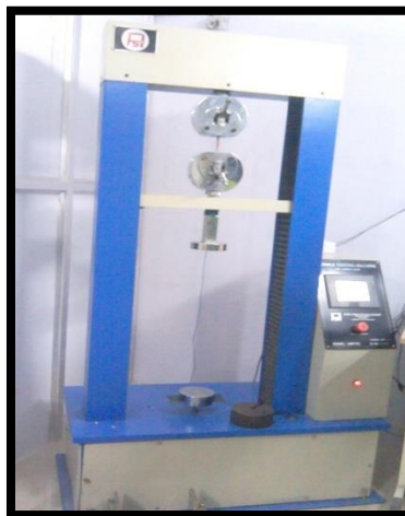
Fig. 3. Universal testing machine
