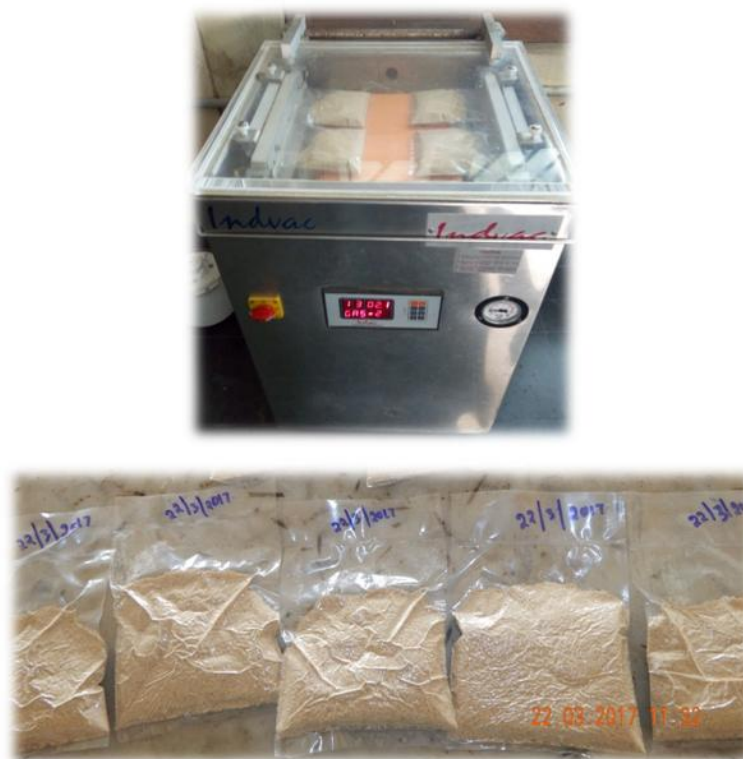
Fig. 1. Vacuum packing of sesame meal and packed sesame meal samples
