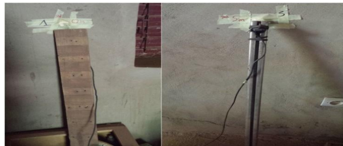
Fig. 9. Images of thermocouples immobilized with wooden and metal tube supports
