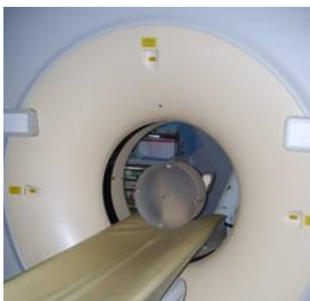
Figure 3. Example of phantom positioning into the CT gantry.
